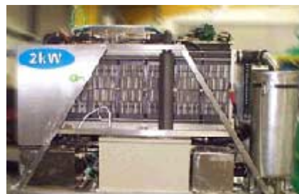
Fig. 11 2kW AFC [Fuel Cell Control Ltd web site]
