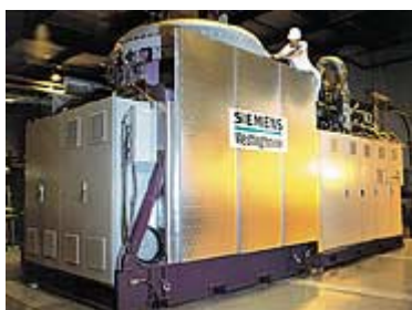
Fig. 14 The Siemens Westinghouse 220kW SOFC-gas turbine hybrid [Siemens web site]
