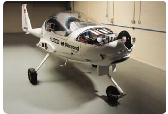
Fig. 40 Intelligent Energy Combined heat and power for the Japanese residential market(left) and fuel cell power train for light aircraft(right) [Intelligent Energy web site]
