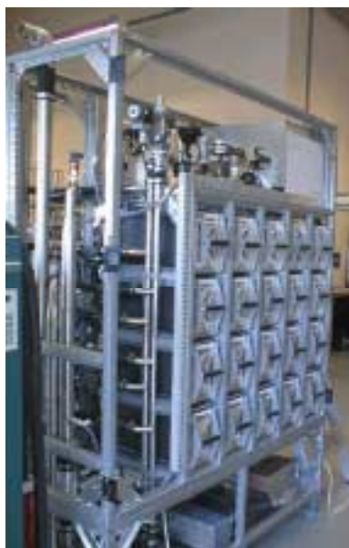
Fig. 41 a 50kW PEMFC CHP unit of IRD Fuel Cells A/S (left) and a 10kW unit the company produced for the Utsira project (right) [IRD Fuel Cells web site]
