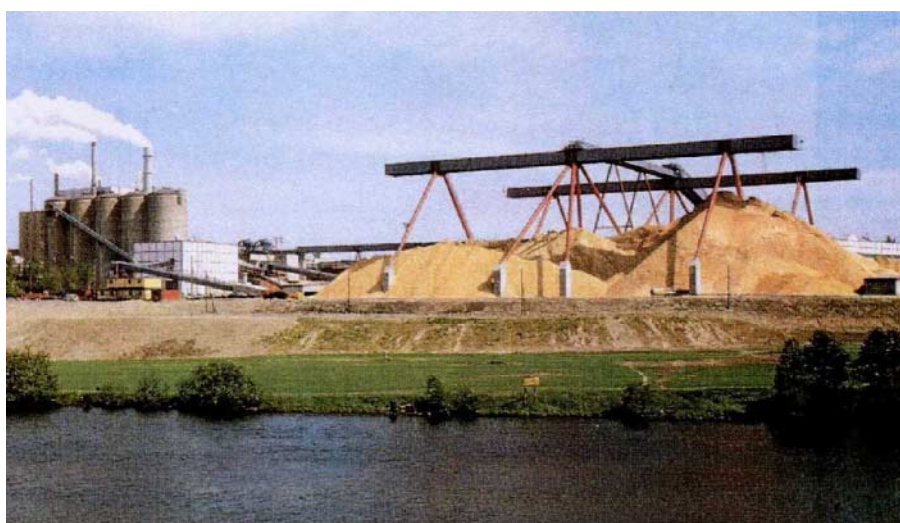
Figure 3. Wood chip stockpile; an increasingly popular feedstock for co-combustion and co-gasification applications
