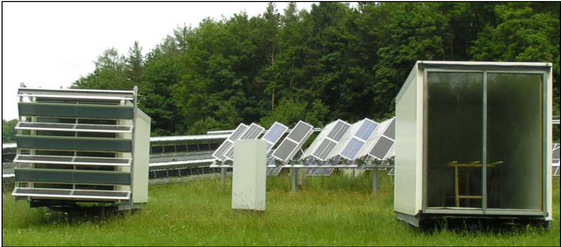
Figure 5: Test containers: CTL PV louvre system with second generation louvres, see Barcelona demonstrator (left) and reference façade (right)
