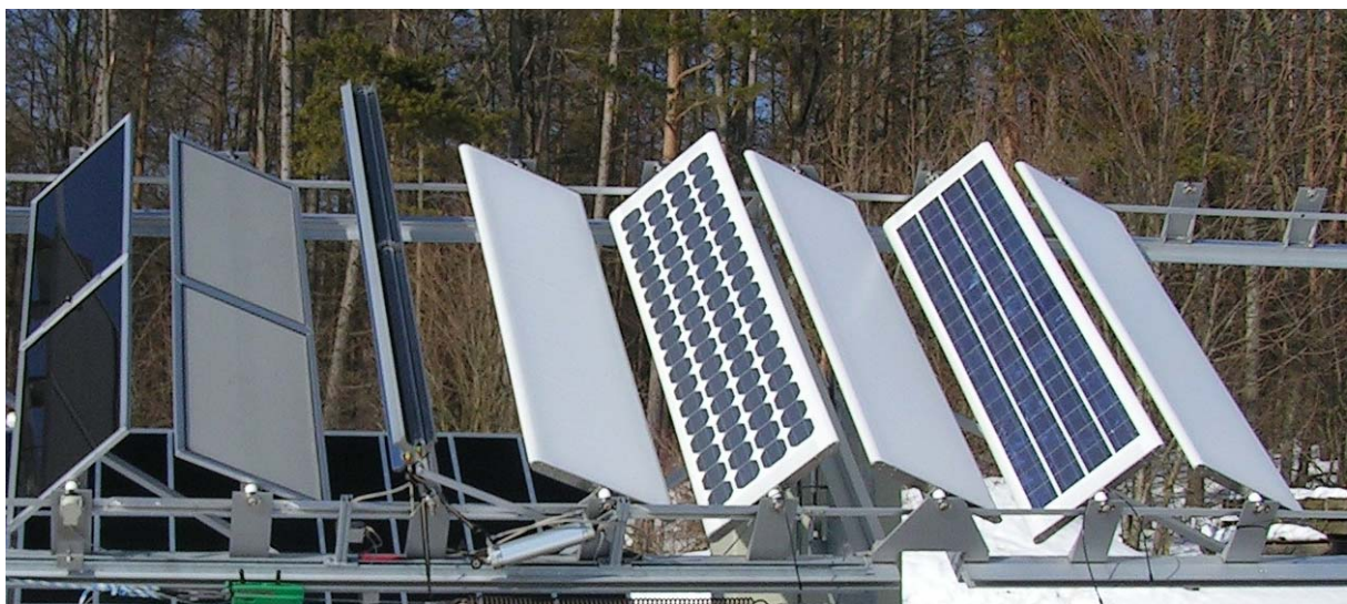
Figure 3: Test stand for louvre sample analysis, first generation louvres (see Paris demonstrator)
