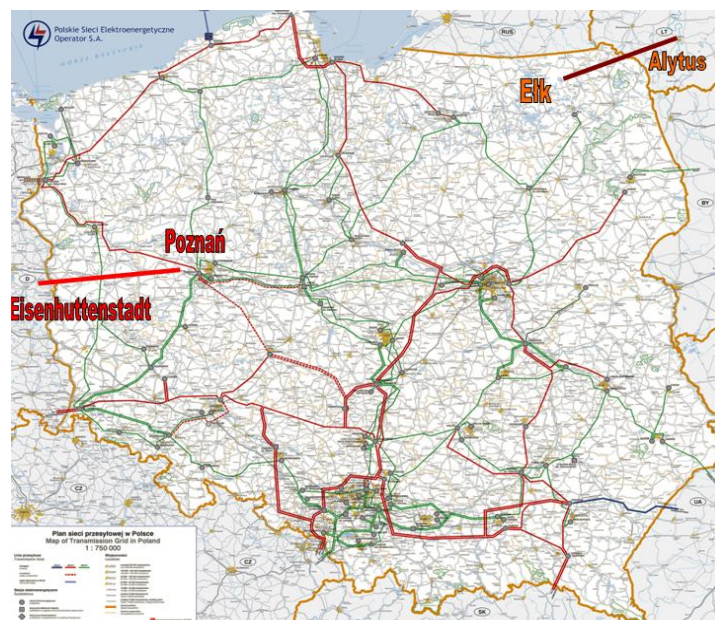
Fig. 1: Two new power lines being the European priority projects and supervised by the European Coordinator.
