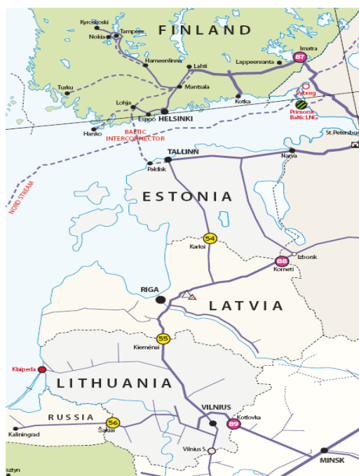
Figure 1: Current gas network within the East-Baltic region
