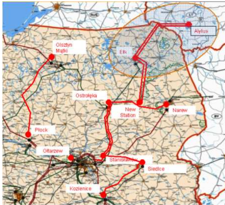
Fig. 5-1 – AC reinforcements needed internal to the Polish grid following the commissioning of the LitPol interconnector
