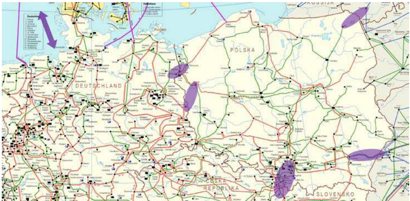
Fig. 6-1 – Interconnection reinforcements proposed at the borders of Germany and Poland in the UCTE Transmission Development Plan [5]
