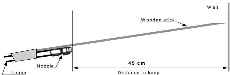
Figure 5.10. Wooden stick fixed on the lance (Lacarin, 1998)
