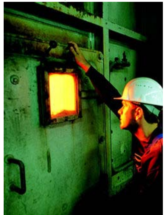
Figure 15: Site visit to the incineration plant of ANO GmbH & Co. KG- Visual Control of the incineration process
