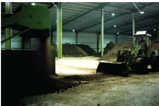
Figure 10: Site visit to Umweltschutz Nord GmbH & Co. - Biological Treatment of oil-contaminated soil in big halls
