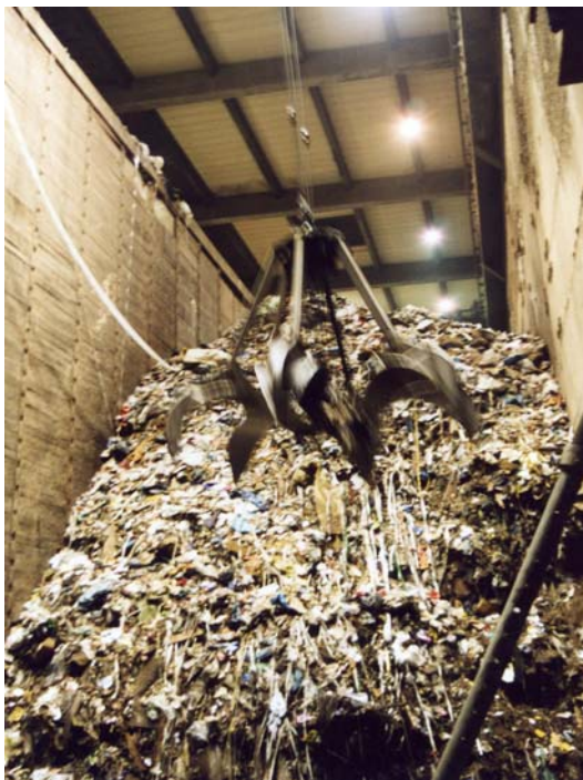
Figure 14: Site visit to the incineration plant of ANO GmbH & Co. KG- Storage area for waste prior incineration
