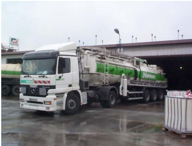
Figure 12: Site visit to company Nehlsen Plump- a special truck for oil-water separation
