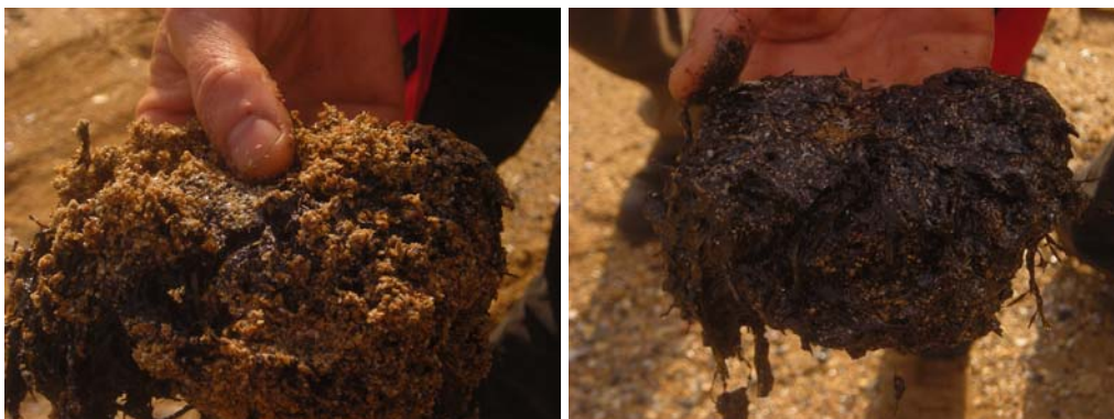
Figure 11 – a) oil/sea-plant/sand mixture; b) oil/sea-plant/sand mixture after washing
