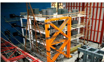
Bi-axial PsD test of a 3-storey asymmetric RC structure
