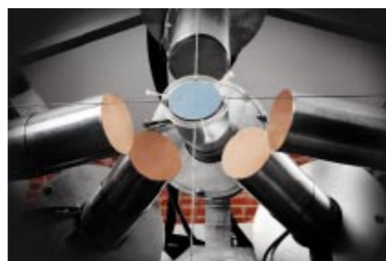
Gamma-ray spectrometer for neutron non-elastic scattering reactions
