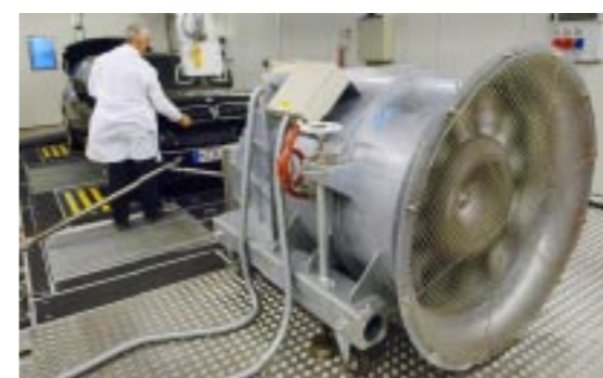
The Vehicle Emissions Laboratory (VELA), operated by the IES and equipped with the most advanced facilities and instrumentation, allows the testing of the emissions from all types of vehicles and automotive fuels.
