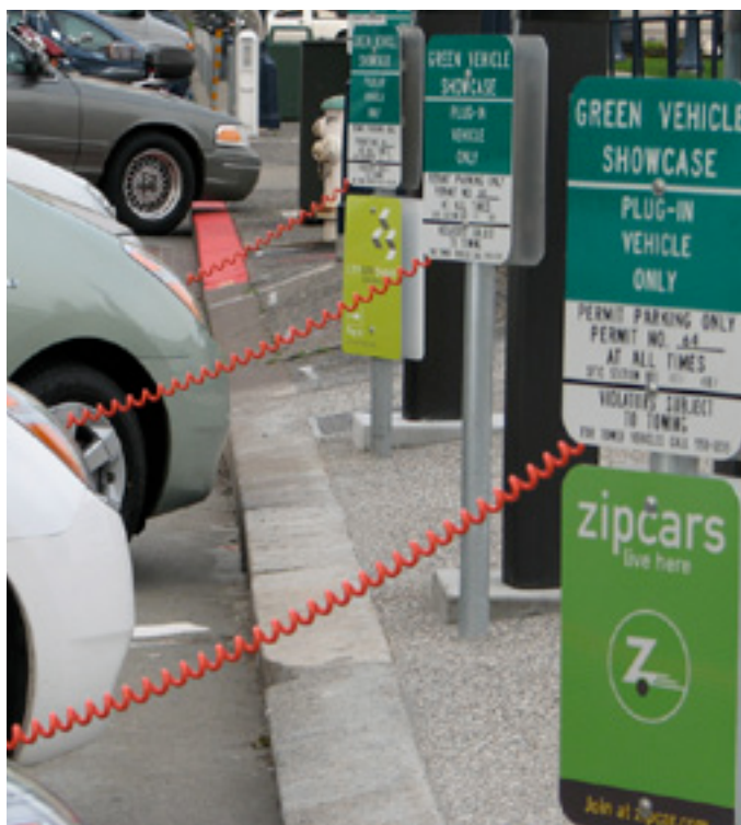
Three plug-in hybrid cars charging at a public recharging station in San Francisco.
