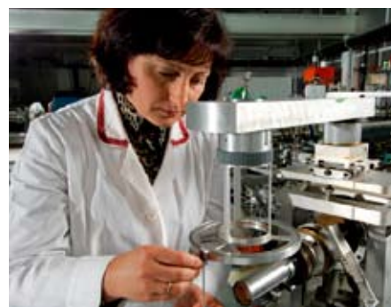
Low-scattering set up for activation studies at JRC-IRMM's Van de Graaff laboratory
