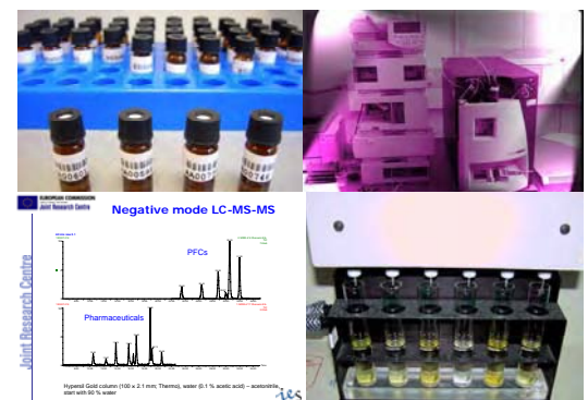
The organic pollutants were analysed by means of HPLC-MS/MS Detection after Solid-Phase Extraction (SPE).
