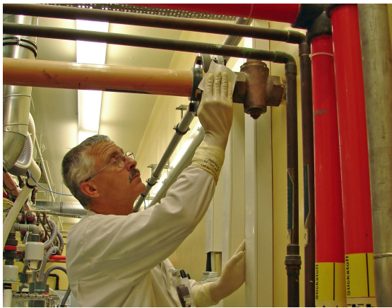
Fig. 1: Swipe sampling technique used to collect dust at a nuclear facility. The sampling locations will differ according to the type of facility that is inspected. Typical sampling locations can be tube connections for UF_6 at enrichment facilities or ventilation conducts. Environmental samples are taken in the search for non-declared nuclear activities or for the verification of declared ones. The samples are either analysed in bulk, giving the average isotopic composition of the material, e.g., uranium, or analysed individually as particles.
