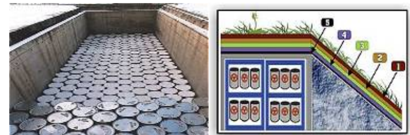
Engineered near-surface disposal
