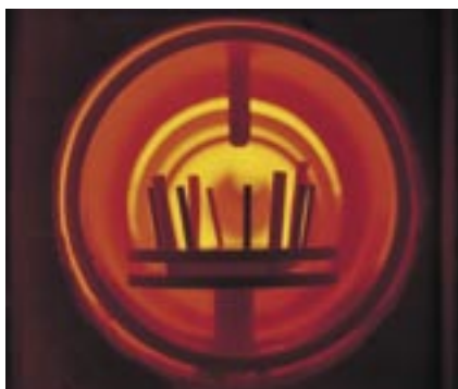
Advanced materials in a laboratory burner rig.
