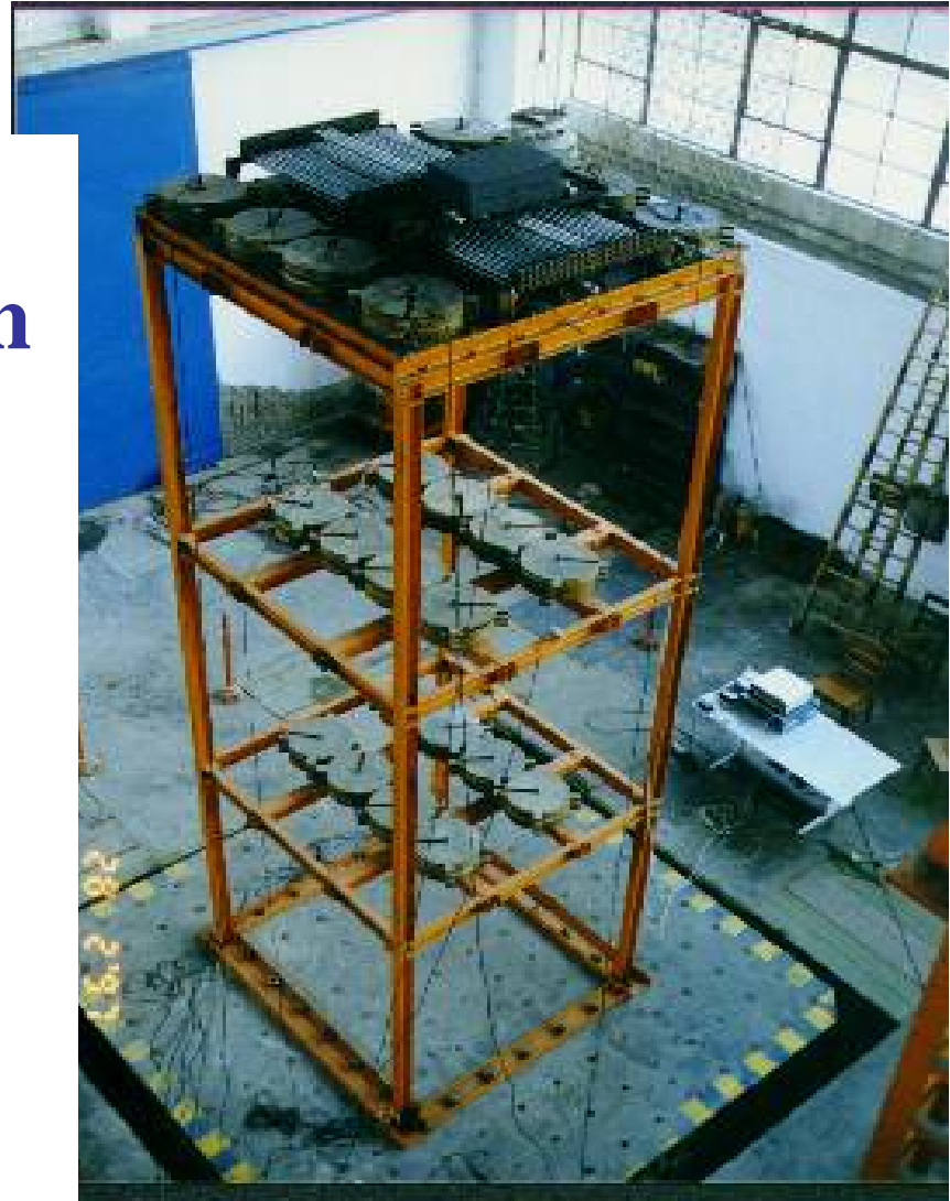
3-story steel frame model in testing
