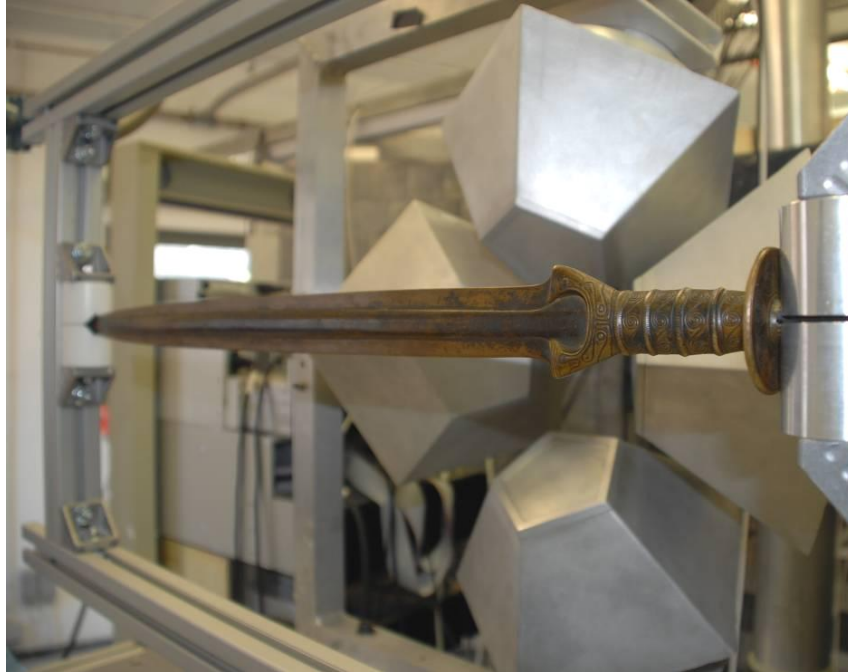
Figure 1. The Buggenum sword, dating from 1300-1100 BC, undergoing measurements at the Joint Research Centre (JRC) in Geel, Belgium. A beam of neutrons was directed onto the sword, and a technique called 'neutron-resonance capture analysis' was used to determine the composition and structure of the Bronze Age artefact.
