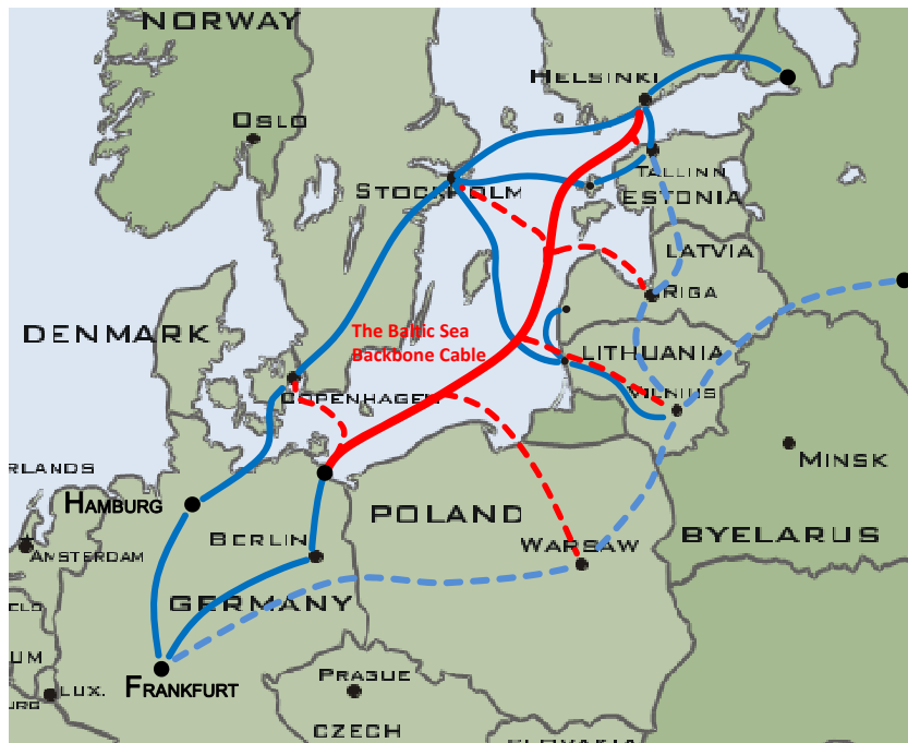
Figure: New Baltic Sea submarine cable (in red) with optional branches to the Baltic Sea countries (red dotted line); current connections to Central Europe (continued blue line); and planned connections (blue dotted line)
