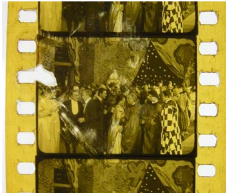
Scratching, base damage
