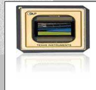
Texas Instruments DMD (Digital Micro-Mirror Devices, 2048x1080).
