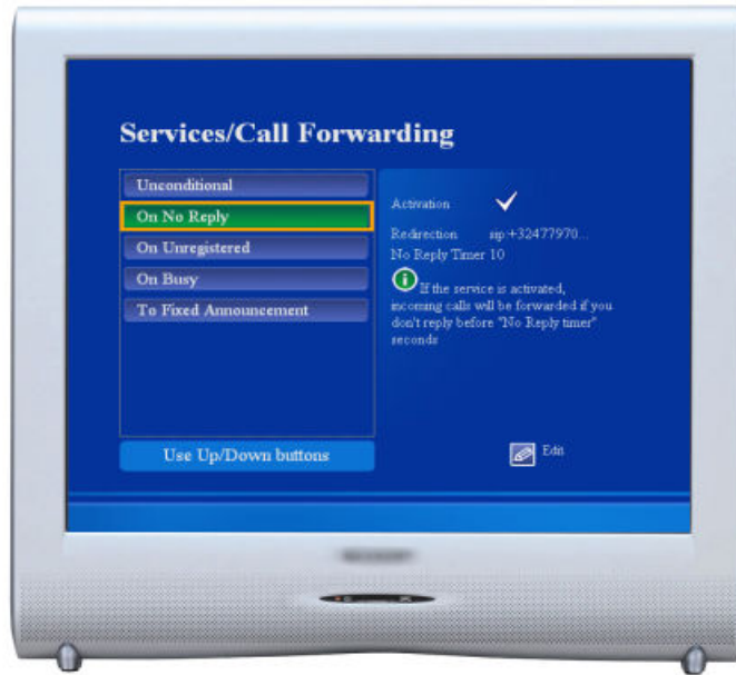
Figure 7: Example of the Call forwarding on No reply settings in the “Services” section
