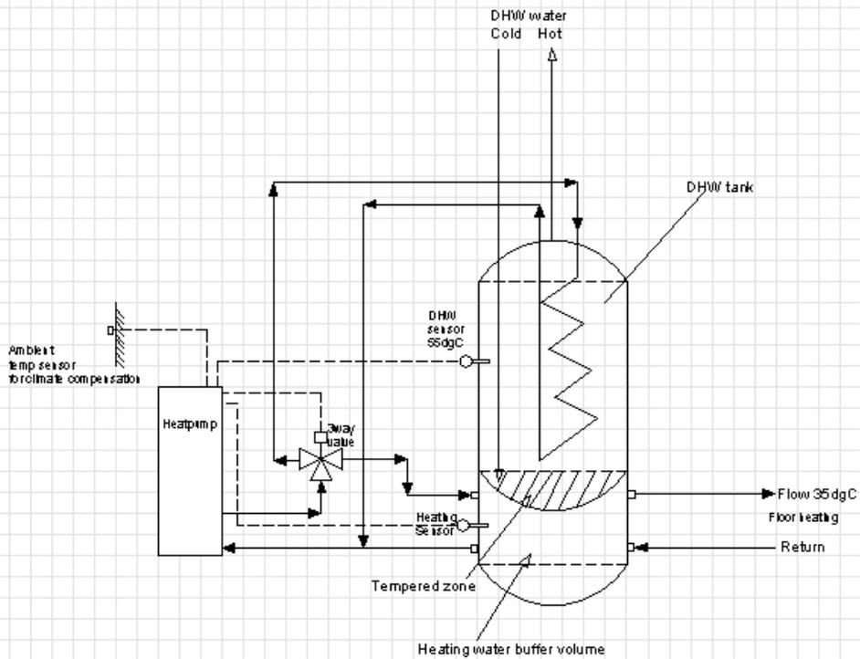
The product is a stand-alone, hot water storage tank, for combined DHW water and heating water. It is designed for use with heat pumps with climate compensation, hot water priority and build-in heating elements for legionella program and backup.
